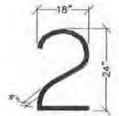
SPECIAL MARKING DETAIL TYPICAL LANE NUMBERING
